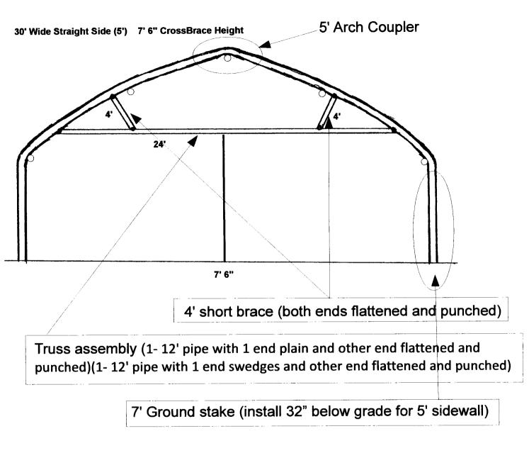
Truss assembly and short braces are to fastened to the bow with brace bands and carriage bolts.
